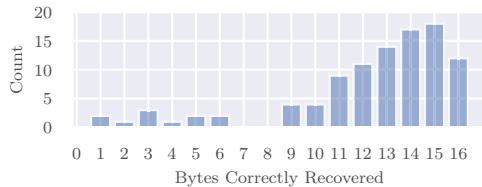
Fig. 2: With the prefetcher enabled, our state recovery technique often only partially recovers the 16-byte AES key. We depict the frequency with which a given number of bytes were recovered, across 100 trials.
